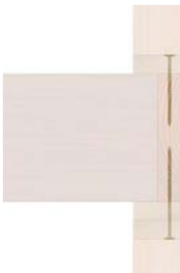
Single 45mm wall plate into side grain.
