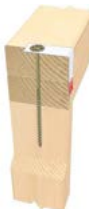
Double 45mm wall plate into end grain.
